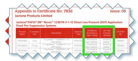
This provision in PAFSS DLP fixed fire suppression systems also future proofs the systems performance against maintenance or modifications that introduce further vent areas or fans to the enclosure that is being protected.
